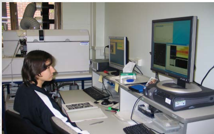
Valeria Murgulov using the Agilent 7500 for U/Pb dating of zircons with the help of the GLITTER software.
