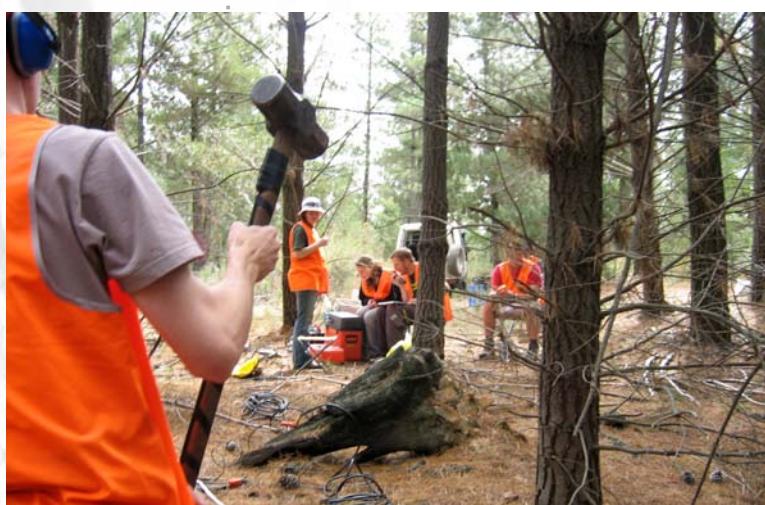
GEOS316 Exploration Geophysics students undertaking a seismic survey using a sledge hammer as a seismic source.
